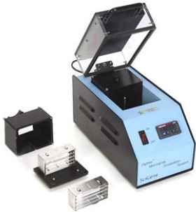
Hybex heating base with microarray chambers and slide racks.
